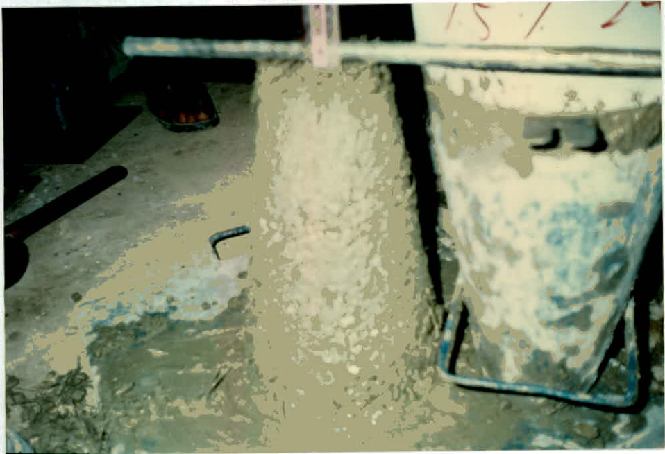
Figure 3.4 : The slump for concrete grade 20 MPa with glass fiber ratio of 1.5% V_f and fiber length of 24mm
