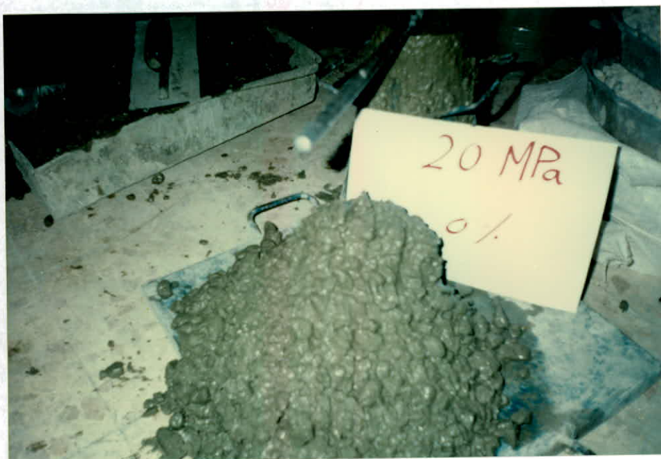
Figure 3.2 : The slump for control mix of concrete grade 20 MPa, collapse slump
