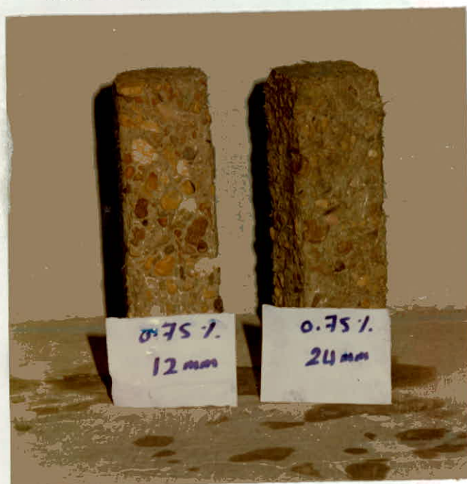
Figure 3.42 : Weight loss after 300 cycles of freezing and thawing for concrete Grade 20mpa and fiber ratio = 0.75\%V_f
