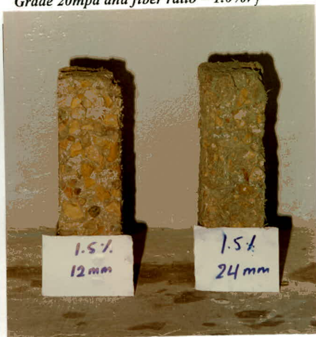
Figure 3.44: Weight loss after 300 cycles of freezing and thawing for concrete Grade 20mpa and fiber ratio = 1.5\%V_f
