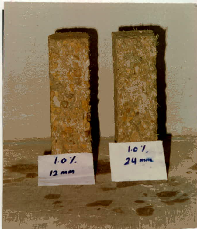
Figure 3.43 : Weight loss after 300 cycles of freezing and thawing for concrete Grade 20mpa and fiber ratio = 1.0\%V_f
