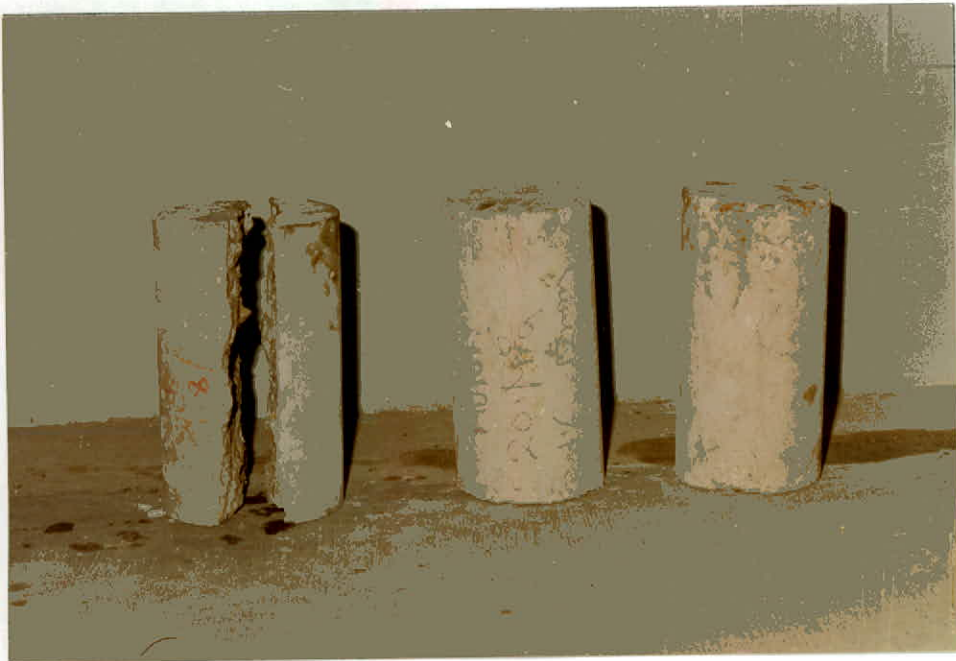
Figure 3.23: The mode of failure for concrete cylinders with and without fiber.
