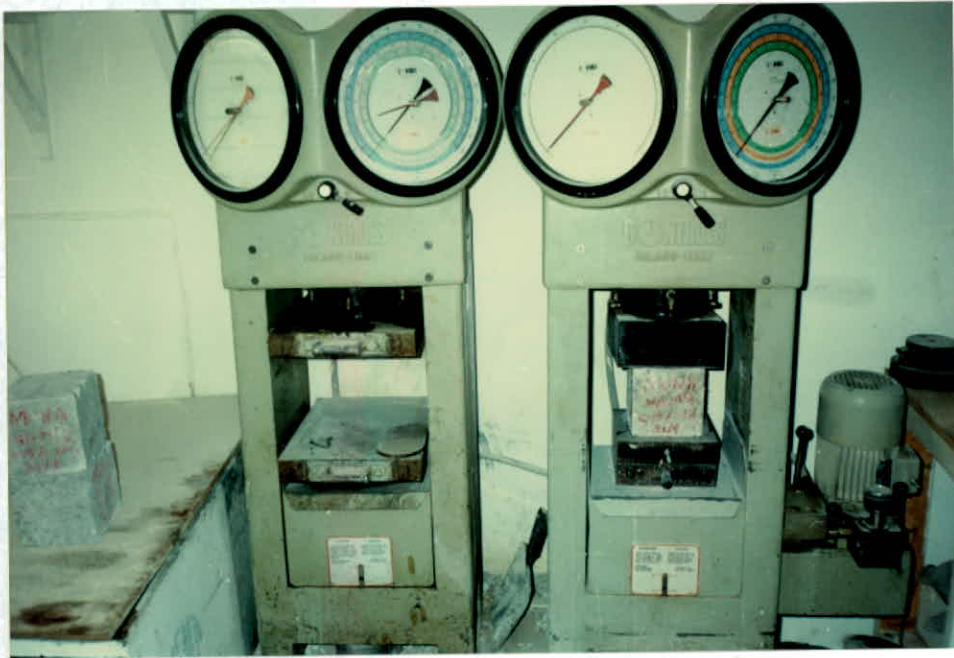
Figure 2.6 : The Compression testing machine, Controls Type.
