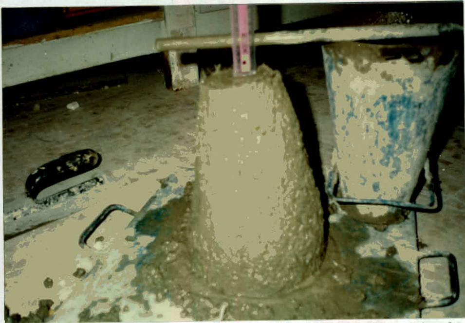
Figure 3.3 : The slump for concrete grade 20 MPa with glass fiber ratio of 0.75% V_f and fiber length of 12mm
